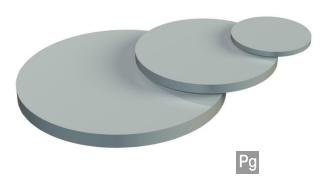
The sealing plate offers both mechanical protection and the maintenance of the protection rating of plastic and metal cable glands to DIN 46320 before cable installation.
