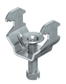
To fasten earthing strips with widths of up to 30 mm to profile rails, suitable for all C profile rails with 16-17 mm slot width.
