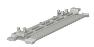
Cover clip for better and easier laying of lines in the WDK trunking. The cover fixing device can be moved along the entire length of the trunking. The cover clip is locked on one side and moved forward. This provides a 30° opening, meaning that cable routing is very simple.
