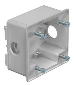
Device socket for mounting CEE sockets in WDK trunking from trunking width 150 mm. The device socket can also be used as a concealed installation socket for CEE devices. Straight version, 16 and 32 A, with 60 x 60 mm hole pattern
