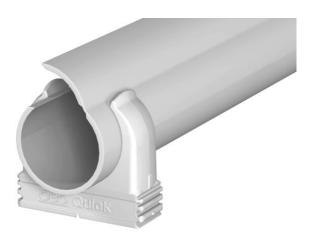
Set consisting of Quick pipe electrical installation pipes and Quick clip surface-mounted clips. For surface-mounted routing of cables in interiors and protected outdoor areas. Universal fastening on wall and ceiling. Comprises 20 m of pipe each of 2 metres in length and 60 Quick clips. Can be used in a temperature range of –25 to +60 °C.
