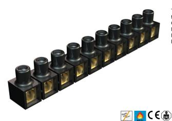
Terminals made of brass, screws of steel, galvanised and transparently passivated, 10-pole, strip separable into individual terminals, open on both sides. Captive upwards screw.
