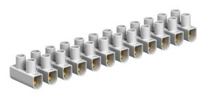
Tested to EN 60998. Steel terminals, steel screws, electrogalvanised, 12-pole, individual terminals detachable from strips using "twist'n'pull". Captive upwards screw. Max. approved ambient temperature to EN 60998: -5 to +80 °C. Nominal cross-section 10 ÷ mm<sup>2</sup>. Nominal voltage 450 V. Nominal current 57 A. Max. attachment each side: 10 mm<sup>2</sup> single-wire or 6 mm<sup>2</sup> multi-wire/flexible.
