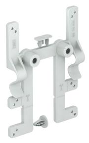
The fastening element BE TS KR can be used to attach OBO junction boxes, type T60 and T100, to all standard cable trays in a few actions, quickly and without tools.
