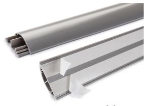
Floor trunking for covered cable routing in internal areas. With snap-on cover and base, with base perforation for direct wall mounting. Change the direction with the fittings and close the trunking ends with end pieces. Service outlet for installing power and data technology.
