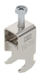
Clamp clip with hammerhead foot, metal pressure sleeve with rounded edges to protect the cable. For vertical and horizontal mounting of 1 single cable on a C-profile rail. For a slot width 16–17 mm. With 1-start screw thread on pressure sleeve, universal hexagonal screw head WAF10, with slot and cross recess. Suitable for assembly indoors and outdoors. We recommend the use of a countersleeve.
