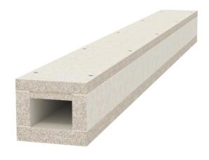
Fire protection duct made from water and frost-proof fibreglass lightweight concrete of building material class A1 according to EN 13501-1 for fireproof laying of photovoltaic cables inside and outside of buildings. The requirements of accidental contact protection for emergency forces are met. Classification I30 as I duct according to DIN 4102 Part 11 for the protection of rescue and emergency routes
