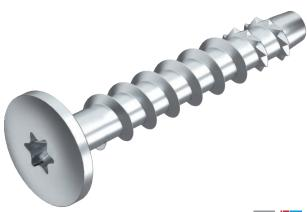
Bolt tie for direct mounting without additional anchors in cracked and uncracked concrete and masonry. With large round head to fasten mounting and profile rails. Torx drive T30.  ${\it Construction product tested according to EAD and CE mark, with European Technical Assessment}$ (ETA) and proof of suitability. Load-bearing capacities under fire loads proven up to fire resistance
