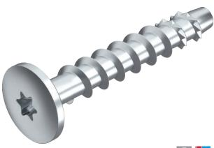
Bolt tie for direct mounting without additional anchors in cracked and uncracked concrete and masonry. With large round head to fasten mounting and profile rails. Torx drive T30.  ${\it Construction product tested according to EAD and CE mark, with {\it European Technical Assessment}}$ (ETA) and proof of suitability. Load-bearing capacities under fire loads proven up to fire resistance
