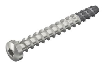
Stainless steel screw-in anchor for direct mounting without additional anchors in cracked and uncracked concrete and masonry. With round head for universal fastenings in wet rooms and outdoor areas. Torx drive T30.
