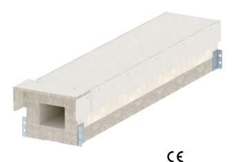
Fire protection duct made of water- and frost-resistant fibre glass lightweight concrete of material class A1 according to EN 13501-1 for fireproof routing of cables in escape and rescue routes. EI90 classification as installation duct according to EN 13501-2 on the basis of tests according to EN 1366-5. When there is an internal fire load (cable fire), the duct prevents the spread of fire from one fire section to another.
