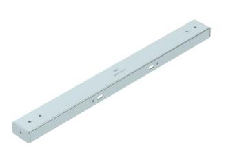
Crossbeam of the symmetrical floor support for the BKRS system, suitable for base type BSSU 190 4060. Can be used for walkable cable trays of width 500 mm. With threaded unions for cut-free mounting of cable trays. Fastening to base with 4x FKS M6 flat-head screws. Fastening material must be ordered separately.
