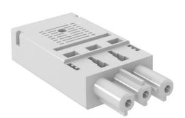
Socket part, 3-pin, type GST18i with spring power connection for rigid cables of 1.5–2.5 mm², single-wire and ultrasonically welded, fine wire cables 1.5 mm² with end sleeves, unmounted with strain relief, can be terminated in situ, 250 V, 16 A.
