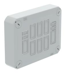
Pluggable cover for the closing of junction boxes, equipped with 8 break-out openings for connection sockets by Wieland and Wago, 3- to 5-pole With quick lock in cover, sealable. Halogen-free material, UV-resistant Flame-resistant to DIN EN 60695/2/11, test temperature 650 °C. Impact resistance IK07 at room temperature. Protection class IP30.
