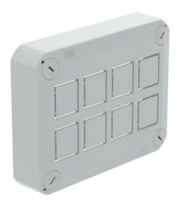
Pluggable cover for the clsoing of junction boxes, equipped with 8 break-out openings for DATA systems based on Keystone. With quick lock in cover, sealable. Halogen-free material, UV-resistant Flame-resistant to DIN EN 60695/2/11, test temperature 650 °C. Impact resistance IK07 at room temperature. Protection class IP30.
