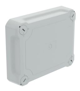
Pluggable cover for the closing of junction boxes, equipped with break-out openings for multiple-pole systems or DATA systems based on Keystone. With quick lock in cover, sealable. Halogen-free material, UV-resistant Flame-resistant to DIN EN 60695/2/11, test temperature 650 °C. Impact resistance IK07 at room temperature. Protection rating IP30
