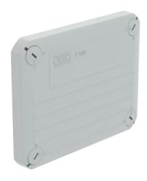
Pluggable cover for the closing of junction boxes, equipped with break-out openings for multiple-pole systems or DATA systems based on Keystone. With quick lock in cover, sealable. Halogen-free material, UV-resistant Flame-resistant to DIN EN 60695/2/11, test temperature 650 °C. Impact resistance IK07 at room temperature. Protection rating IP30
