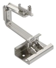
Roof hook to mount photovoltaic modules on pitched roofs in combination with the TP 45 support profile. Suitable for tiled roofs. Lockable fastening on support profile. Mounting on rafters with TKS wafer-head screws. Roof hook can be infinitely adjusted horizontally and vertically using glands, correct spanner Torx 40. Height adjustment in the range of the roof slat between 40–54 mm, side adjustment option up to 76 mm, height adjustment of the support profile up to 18 mm.
