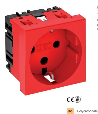
Protective contact socket Single 0°, encoded version, with increased touch protection, with screwless terminals, 2-pin, 16 A, 250 V $\sim$ , with connection terminals according to IEC 60884-1. The socket can only be used in connection with an encoding pin of type CST-STD.
