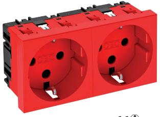
Protective contact socket Double 0°, encoded version, with increased touch protection, with screwless terminals, 2-pin, 16 A, 250  $V^\sim$ , with connection terminals according to IEC 60884-1. The socket can only be used in connection with an encoding pin of type CST-STD.
