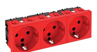
Protective contact socket Triple 0°, encoded version, with increased touch protection, with screwless terminals, 2-pin, 16 A, 250 V $^\sim$ , with connection terminals according to IEC 60884-1. The socket can only be used in connection with an encoding pin of type CST-STD.
