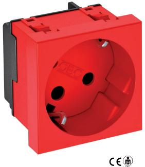
Protective contact socket Single 33°, encoded version, with increased touch protection, with screwless terminals, 2-pin, 16 A, 250 V  $^\sim$ , with connection terminals according to IEC 60884-1. The socket can only be used in connection with an encoding pin of type CST-STD.
