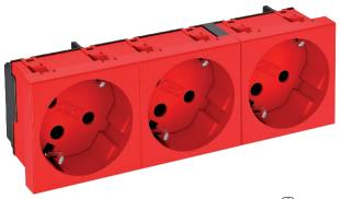
Protective contact socket Triple 33°, encoded version, with increased touch protection, with screwless terminals, 2-pin, 16 A, 250  $V^\sim$ , with connection terminals according to IEC 60884-1. The socket can only be used in connection with an encoding pin of type CST-STD.
