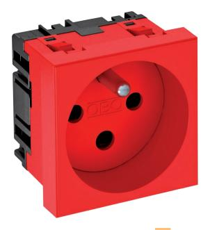
Socket with earthing pin, single 0°, encoded version, with increased touch protection, with screwless terminals, 2-pin, 16 A, 250 V $^\sim$ , with connection terminals according to IEC 60884-1. The socket can only be used in connection with an encoding pin of type CST-STD.
