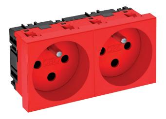
Socket with earthing pin, double 0°, encoded version, with increased touch protection, with screwless terminals, 2-pin, 16 A, 250 V $^{\sim}$ , with connection terminals according to IEC 60884-1. The socket can only be used in connection with an encoding pin of type CST-STD.
