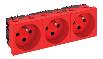
Socket with earthing pin, triple 0°, encoded version, with increased touch protection, with screwless terminals, 2-pin, 16 A, 250  $V^\sim$ , with connection terminals according to IEC 60884-1. The socket can only be used in connection with an encoding pin of type CST-STD.
