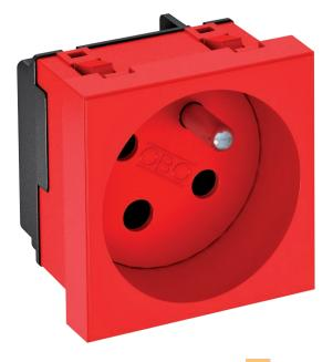
Socket with earthing pin single 33°, encoded version, with increased touch protection, with screwless terminals, 2-pin, 16 A, 250 V  $\widetilde{\phantom{a}}$ , with connection terminals to IEC 60884-1. The socket can only be used in conjunction with an encoding pin, type CST-STD.
