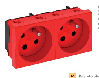
Socket with earthing pin double 33°, encoded version, with increased touch protection, with screwless terminals, 2-pin, 16 A, 250 V $^{\sim}$ , with connection terminals to IEC 60884-1. The socket can only be used in conjunction with an encoding pin, type CST-STD.
