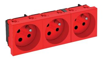
Socket with earthing pin triple 33°, encoded version, with increased touch protection, with screwless terminals, 2-pin, 16 A, 250 V  $\widetilde{\phantom{a}}$ , with connection terminals to IEC 60884-1. The socket can only be used in conjunction with an encoding pin, type CST-STD.
