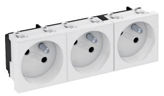
Socket with earthing pin Triple 33°, with increased touch protection, with screwless terminals, 2-pin, 16 A, 250V  $^\sim$ , with connection terminals to IEC 60884-1.
