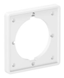
Intermediate flange for 16 A and 32 A CEE sockets. Also contained in type CEE16E2 and CEE32E2 for Rapid 80 and ISS). Is used as a frame when mounting the CEE mounting box. For installation in Rapid 80 device installation trunking and ISS service poles.
