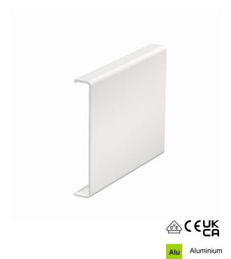
Aluminium cover, for closing Rapid GA device installation trunking and ISS service poles with a 76.5 mm system opening. The firm position of the cover and electrical contact to the lower part of the trunking and service pole is guaranteed thanks to type RKV3V locking brackets. There are 2 pre-mounted locking brackets included per delivery length (100 mm).
