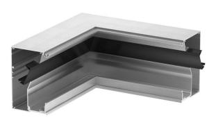
Internal corner base to create a design device installation trunking of the GAD series. 45 mm system opening for acceptance of Modul 45 switch and connection devices and appropriate PVC and aluminium covers of the Rapid 45 series. The fitting can be completed with fitting covers in the "Swing", "Soft" or "Style" design. The GAD OTA cover adapters are essential. A GAD OTD spacer must be placed between the trunking covers.
