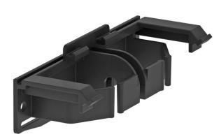
Cover adapter for mounting on trunking bases and fittings of the GAD and Rapid IBIS design device installation trunking series. The cover adapter can be pushed into a guide on the base and is used to accept the trunking cover and keep it at the desired spacing. It is also used for bundled cable exits and can be moved into the lengthwise direction. A maximum spacing of 500 mm between the cover adapters must be maintained.
