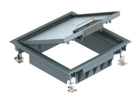
Service unit for 4 installation devices in 2 UT universal supports for use in raised floors for indoor use. Fastening bracket in a clamping range of up to 50 mm plate thickness
