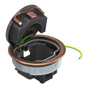
Round installation unit with floor covering protection frame for direct installation in the connection socket UDL2-120 for indoor use. When closed, the installation unit can be wet-cleaned. The minimum installation depth is 70 mm.
