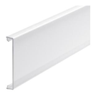
Trunking cover for closing Rapid 80 GK (PVC), GS (steel) and GA (aluminium) device installation trunking as well as ISS service poles with a 76.5 mm system opening. The GK-OTGO cover is made from translucent but milky plastic (looking like cut glass) and is therefore suitable for integrating lighting in the trunking or service poles.
