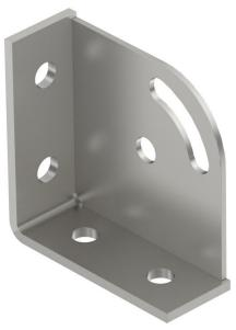
Reinforced mounting bracket with 6 holes to connect profile rails 41 x 41 mm and 41 x 21 mm at an angle of 90°. Additional fastening option for a strut at an angle of 45° with an adjusting range of +/- 30°. Can be used for angles between 15° and 75°.
