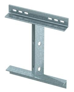
Adapter plate with slots for universal fastening to vertical steel girders and walls. Wall and support brackets are screwed to the adapter plate at a 45° angle. To support cable support systems in building corners and jumps. The hexagonal bolts, type SKS 12 x 40 GF, are used to fasten the brackets to the adapter plate. Please order the appropriate quantity.
