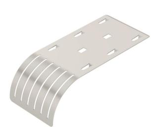
Drop-out plate for mesh cable trays. The exit plate allows compliance with specific bend radii, thus preventing possible cable breaks. Can be mounted in a lengthwise direction and at the side, can be arranged for greater widths.
