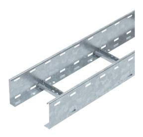
Cable ladder with 110 mm side height with welded C30 profile rungs which are open in an upwards direction. Rolled side rail for reinforcement and as edge protection. Fastening to the bracket takes place using clamps, type LKS 40. The slot dimension of the frame is 16.5 mm and the appropriate clamp clip is type 2056.
