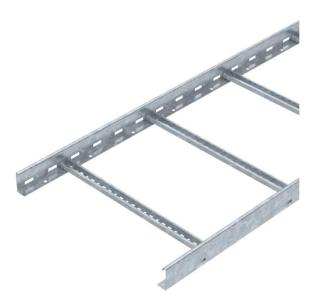
Cable ladder with a 60 mm side height with welded C30 profile rungs which are open in an upwards direction. Rolled side rail for reinforcement and as edge protection. Fastening to the bracket takes place using hold-down clamps, type LKS 40. The slot dimension of the rung is 16.5 mm and the appropriate clamp clip is type BS-H....
