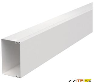
Trunking cover and base with base perforation. Equipotential bonding is guaranteed between the cover and the base without any additional aids. The LKM cable trunking, type LKM 60100FS, has been tested for the maintenance of electrical function as a routing system according to DIN 4102 Part 12. Please note the cable types tested in the BSS fire protection systems division!
