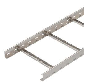
Cable ladder with perforated side rail of side height 60 mm with riveted C profile frames, open in an upwards direction (VS version).
