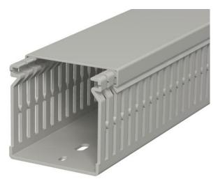
Wiring duct, incl. cover and base perforation, for horizontal and vertical routing of electrical cables in the switchgear cabinet. Designed as a metric duct. The nominal dimension of the system size corresponds to the internal dimension of the duct. Retainers are broken out without tools. The flush-floor routing of cables is possible through predetermined break points. Tapering in the side slots prevents the cables from falling out. Tested to DIN EN 50085-2-3. Special lengths on request.
