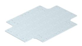
This mounting and fastening plate gives the options for variable fixing of external components in the junction box. It consists of strip-galvanised sheet steel of a material thickness of 2 mm.
